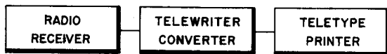
BLOCK DIAGRAM EQUIPMENT NEEDED TO RECEIVE RADIO TELETYPEWRITER FSK OR AFSK SIGNALS
